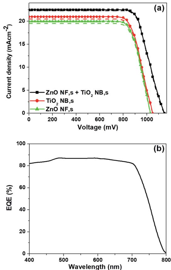
Fig. 5  $J$ - $V$  curves of (a) best performing PSCs based on three different ETMs both in the forward and backward scans, and (b) EQE spectra of the champion devices based on the hybrid ETM, respectively.
