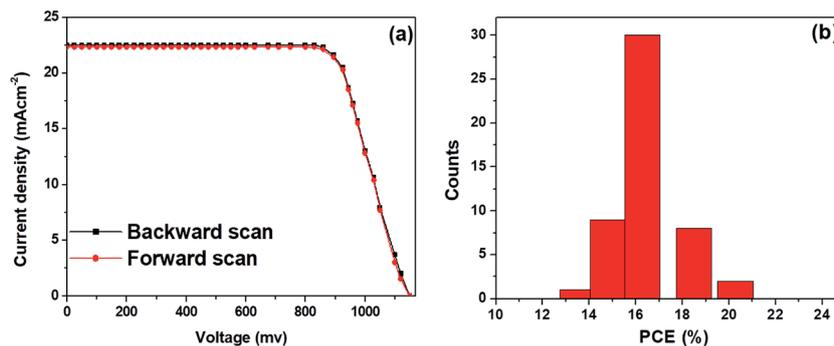
Fig. 6 (a)  $J$ - $V$  curves of the best performing PSCs with the hybrid ETM obtained by forward and backward scans, and (b) PCE distributions for the 50 devices of the corresponding ETM, respectively.
