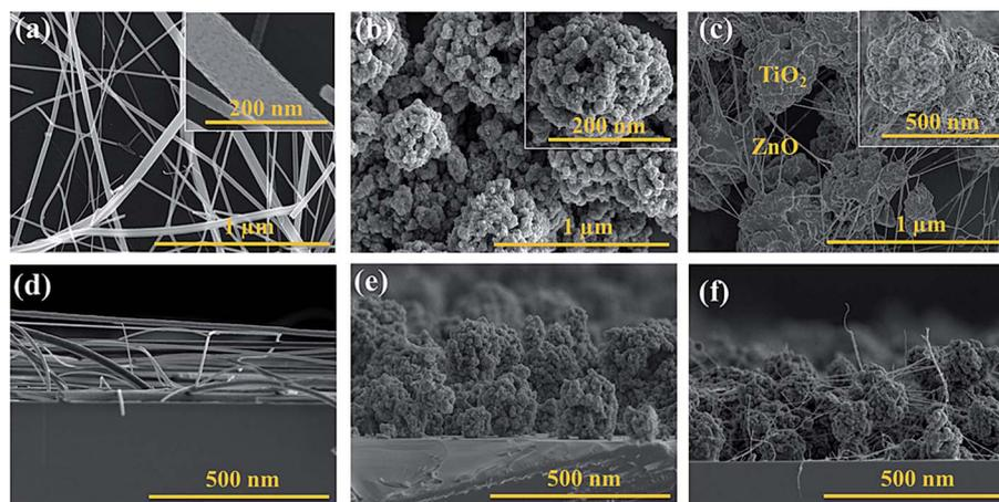
Fig. 2 High resolution surface SEM images of (a) ZnO NFs: inset shows the magnified image of each nanofiber, (b) TiO<sub>2</sub> NBs: inset shows the magnified view of individual nanobeads, (c) blend of ZnO NFs and TiO<sub>2</sub> NBs; inset displays the magnified view of nanobeads surrounded by nanofibers and cross-sectional SEM images of (d) ZnO NFs, (e) TiO<sub>2</sub> NBs, and (f) hybrid ETM of ZnO NFs and TiO<sub>2</sub> NBs, respectively.
