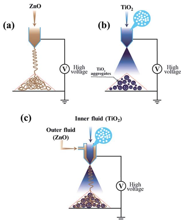
Fig. 1 Schematic diagram of (a) e-spray process for ZnO nanofiber preparation, (b) formation of  $\text{TiO}_2$  nanobeads using e-spraying, and (c) co-axial e-spray process for the formation of hybrid films.
