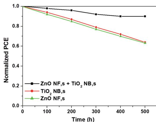
Fig. 7 Long-term stability testing for three different ETMs.
