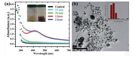
Fig. 1 (a) UV-vis spectra of Ag NPs with the Fagonia cretica extract at different time points (the inset shows the colour change before and after Ag ion reduction) and (b) TEM image of Aq NPs, while the inset shows the particle size distribution.
