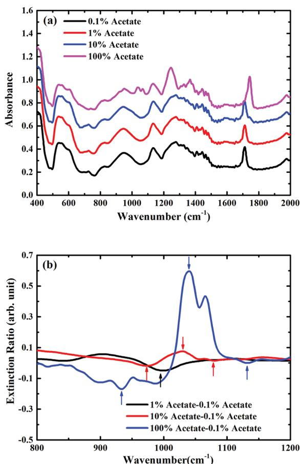
Fig. 6 (a) Measured absorption spectra of mixtures in the presence of metasurface on  $\text{SiO}_2/\text{Si}$  substrate in the ambient atmosphere, spectra are consecutively shifted by 0.2 vertically for clarity; (b) zoomed extinction spectra of mixtures in the presence of metasurface on  $\text{SiO}_2/\text{Si}$  substrate for the carbon–oxygen stretching band region between  $800\text{ cm}^{-1}$  and  $1200\text{ cm}^{-1}$ .
