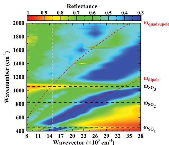
Fig. 3 Simulated dispersion diagram of metasurface on  $\text{SiO}_2/\text{Si}$  substrate. The two red dashed lines show the calculated resonance frequencies (dipole mode and quadrupole mode) of the uncoupled metasurface. The three black dashed lines represent the frequencies of three surface optical phonon modes in  $\text{SiO}_2$ . The vertical white line represents the spectral response of the metasurface on  $\text{SiO}_2/\text{Si}$  substrate presented in this paper.
