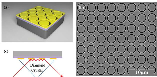
Fig. 1 (a) Schematic diagram of the metasurface design on the  $\text{SiO}_2/\text{Si}$  substrate; (b) top-view SEM image of a  $50\ \text{nm}$ -thick metasurface deposited on the substrate; (c) a schematic illustration of the ATR sampling technique in the measurement.
