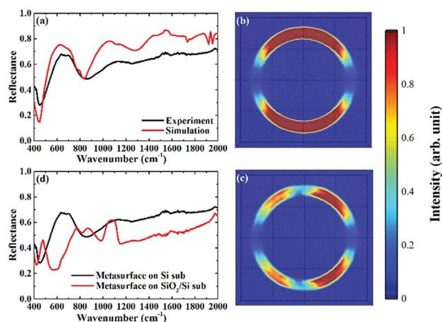
Fig. 2 (a) Measured and simulated spectra of metasurface on Si substrate; (b) electric field distribution for  $x$ - $y$  plane at  $450\ \text{cm}^{-1}$  (dipole mode); (c) electric field distribution for  $x$ - $y$  plane at  $860\ \text{cm}^{-1}$  (quadrupole mode); (d) comparison between metasurface on Si substrate (black line) and on  $\text{SiO}_2/\text{Si}$  substrate (red line).
