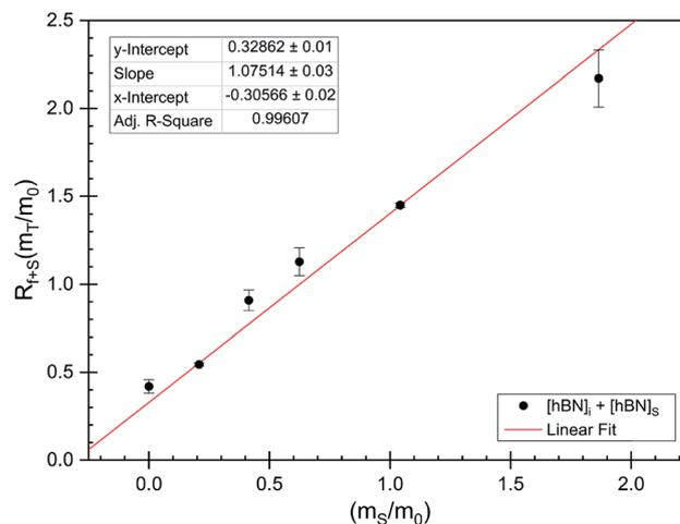
Fig. 4 FTIR peak ratios (out-of-plane/in-plane (R/TO) h-BN stretches) of “spiked” samples are plotted *versus* the ratio of h-BN standard added to the as-received BNNTs per eqn (5). The data is fit using non-linear least squares regression (red line) and the x-intercept is used to determine the h-BN concentration in the initial as-received BNNT sample per eqn (6).
