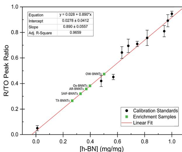
Fig. 5 Calibration curve generated from “spiked” standards after determination of [hBN]<sub>i</sub> in AR-BNNTs. Black circles represent calibration standards. Green squares represent enrichment samples and the calculated weight percent from R/TO peak ratios and based on linear best fit (red line) to calibration curve.
