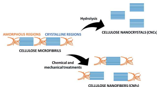
Fig. 3 Production of CNCs and CNFs from cellulose.
