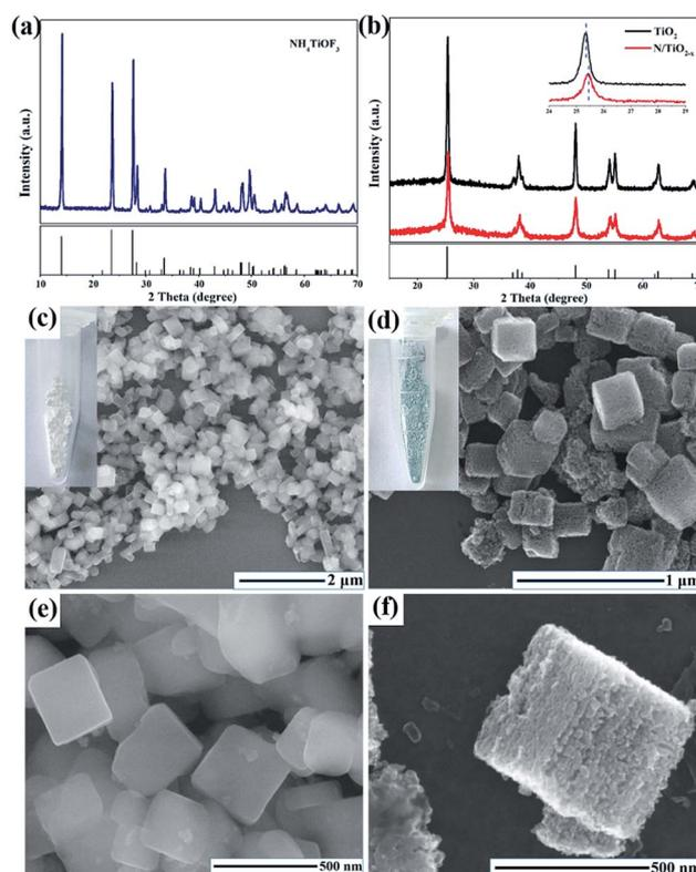
Fig. 1 Schematic representation for the synthesis of TiO<sub>x</sub> nanosheets. XRD pattern of (a) NH<sub>4</sub>TiOF<sub>3</sub> and (b) N/TiO<sub>2-x</sub>, SEM images of (c, e) NH<sub>4</sub>TiOF<sub>3</sub> and (d, f) N/TiO<sub>2-x</sub>.
