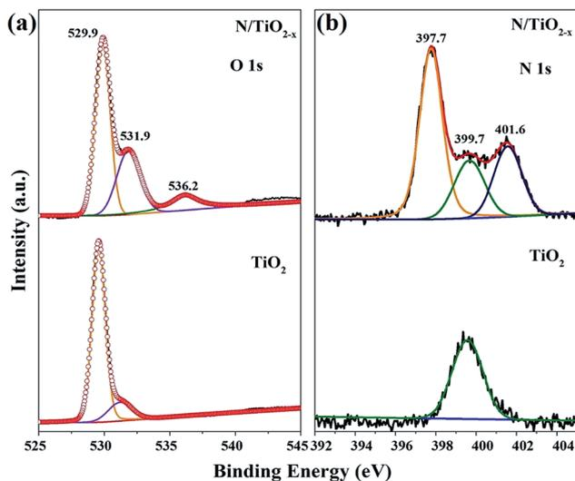
Fig. 4 XPS spectra and fitted data of the as-obtained TiO<sub>2</sub>: (a) O 1s and (b) N 1s.
