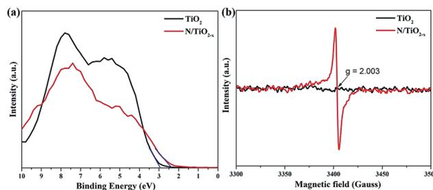
Fig. 5 (a) Valence band XPS spectra and (b) ESR spectra at room temperature of N/TiO<sub>2-x</sub> and unreduced TiO<sub>2</sub> samples.
