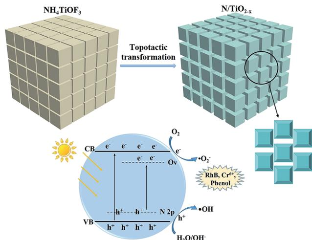
Fig. 8 Schematic of the topological transformation process, and energy band diagrams of the N/TiO<sub>2-x</sub> sample.
