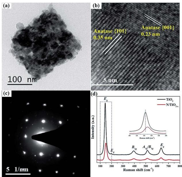
Fig. 2 (a) TEM, (b) HRTEM and (c) SAED patterns of N/TiO<sub>2-x</sub>, respectively, (d) Raman spectra of N/TiO<sub>2-x</sub> and unreduced TiO<sub>2</sub>.
