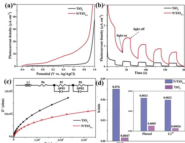
Fig. 7 (a) Linear sweep voltammograms, (b) chronoamperometry tests, (c) Nyquist plots of electrochemical impedance and (d) the reaction kinetics constant of N/TiO<sub>2-x</sub> and unreduced TiO<sub>2</sub> samples under visible light illumination.
