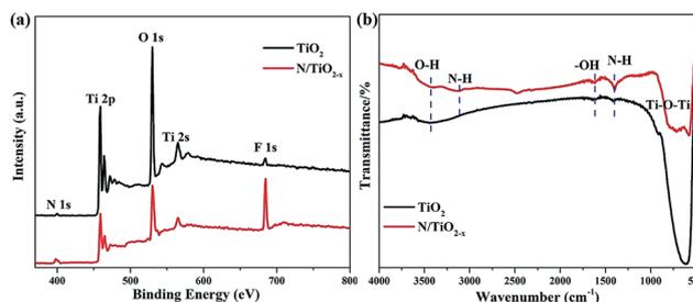
Fig. 3 (a) XPS spectra and (b) FTIR spectra of N/TiO<sub>2-x</sub> and unreduced TiO<sub>2</sub>.
