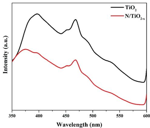
Fig. 6 PL spectra of N/TiO<sub>2-x</sub> and unreduced TiO<sub>2</sub> samples.
