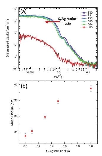
**Fig. 6** (a) Scattering profiles of the *ex situ* AgNP suspension samples with S/Ag ratio of 0 (EB0), 0.1 (EB1), 0.3 (EB2), 0.5 (EB3), 1.0 (EB4), and 5.0 (EB5), respectively. (b) The dependence of mean size of the *ex situ* AgNP samples EB0-EB4 on the S/Ag molar ratio.
