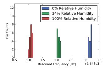
Fig. 5 Resonant frequency of a cantilever is shown for relative humidity values of 0, 34, and 100 percent (cantilever dimensions are: 3 mm long, 100 μm wide, 64 μm high, and a carbon infiltration time of 6 minutes). This histogram shows observations taken while humidity values were sequentially changed in a randomized order. Shifts on the order of 1 Hz were seen on top of a base resonant frequency of 1.65 kHz.
