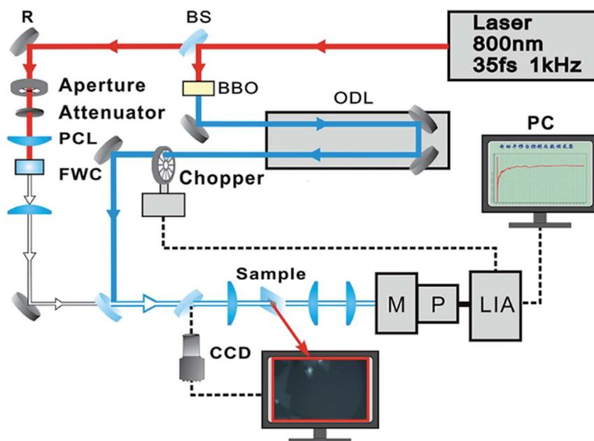
Fig. 2 The schematic diagram of a femtosecond transient absorption spectroscopy system: BS<sub>1</sub> and BS<sub>2</sub>, 3 : 7 and 1 : 1 beam splitter; BBO, 0.5 mm-thick  $\beta$ -BaB<sub>2</sub>O<sub>4</sub> crystal; OD, optical delay line; R, reflector; CL, convex lens; FWC, flow water cell; M, three grating monochromator; P, photomultiplier; LIA, lock-in amplifier.
