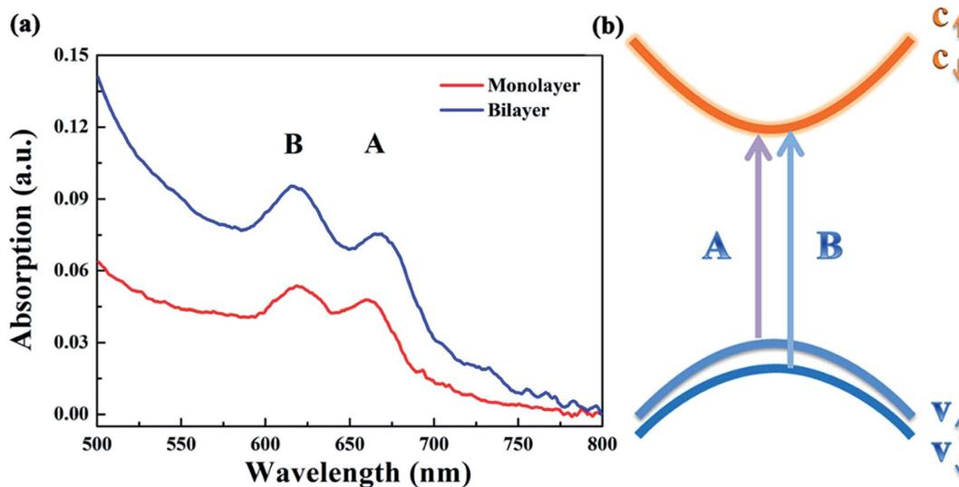
Fig. 4 (a) The UV-vis absorption spectra of the as-grown monolayer and bilayer MoS<sub>2</sub> after being returned to zero at 800 nm; (b) simplified band structure of MoS<sub>2</sub> at the K point in the Brillouin zone.
