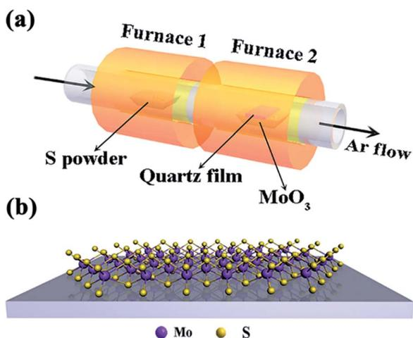
Fig. 1 (a) Schematic illustration of the tube-furnace setup employed in this study for the synthesis of monolayer and bilayer MoS<sub>2</sub>; (b) a schematic view of the two-dimensional structures of monolayer MoS<sub>2</sub> on the substrate.
