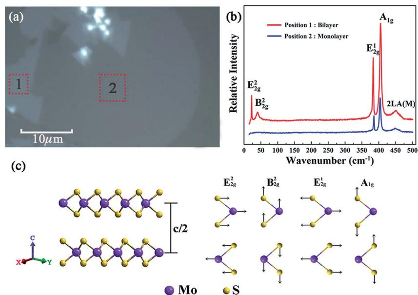
Fig. 3 (a) Optical micrograph of layered MoS<sub>2</sub> samples deposited on the quartz substrate; (b) Raman spectra of the as-synthesized MoS<sub>2</sub> samples in the regions marked '1' and '2' in (a); (c) schematic diagrams of the lattice structure (left side) in out-of-plane directions of MoS<sub>2</sub> and its corresponding characteristic Raman vibration modes (right side).
