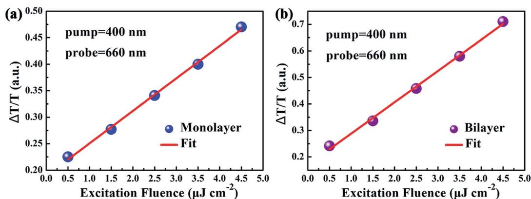
Fig. 5 Signal intensity of  $\Delta T/T$  at zero time delay as a function of excitation intensity for (a) monolayer and (b) bilayer MoS<sub>2</sub> with a pump wavelength of 400 nm and a probe wavelength of 660 nm. The circles denote the experimental data, while the solid lines denote the linear fitting data.
