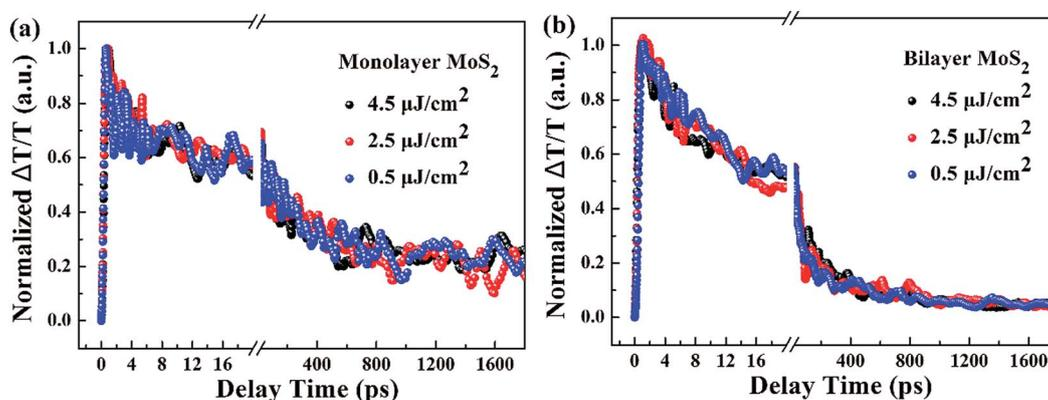
Fig. 7 Normalized transient absorption decay dynamics curves of (a) monolayer and (b) bilayer MoS<sub>2</sub> with a pump wavelength of 400 nm and a probe wavelength of 660 nm at different pump intensities.
