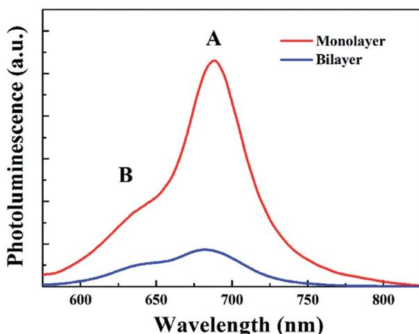
Fig. 8 Photoluminescence (PL) spectra of monolayer and bilayer MoS<sub>2</sub>.
