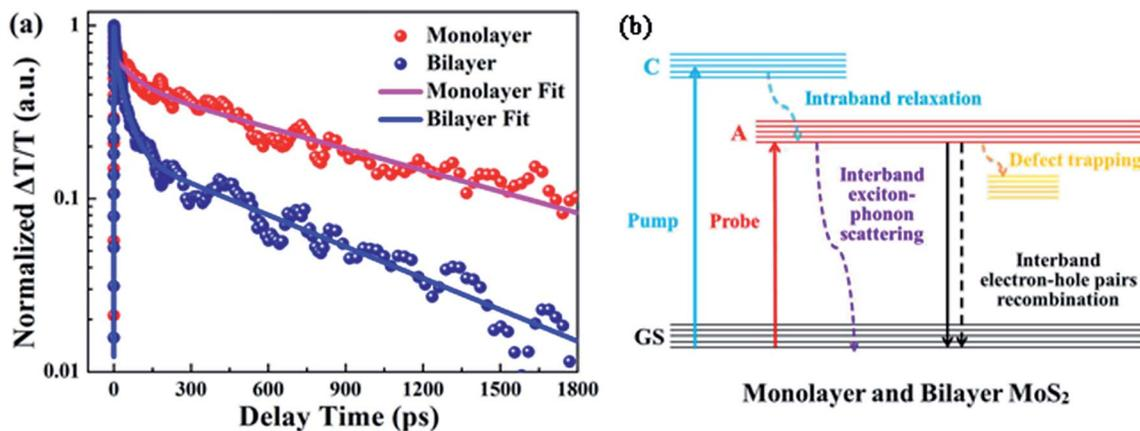
Fig. 6 (a) Experimental (solid circles) and fitted (thick lines) data for normalized transient absorption relaxation dynamics curves of monolayer and bilayer MoS<sub>2</sub>. All the relaxation dynamics curves were normalized at time zero, being fitted with a three exponential function  $I(t) = a_1 \exp(-t/\tau_1) + a_2 \exp(-t/\tau_2) + a_3 \exp(-t/\tau_3)$ ; (b) schematic summary of relaxation processes in monolayer and bilayer MoS<sub>2</sub>.
