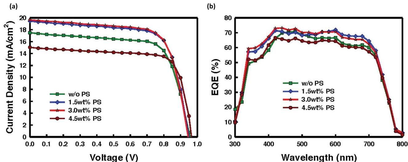
Fig. 2 Device performance of perovskite solar cells with different concentrations of polystyrene (ITO/PEDOT:PSS/CH<sub>3</sub>NH<sub>3</sub>PbI<sub>3</sub> (without or with 1.5, 3.0, 4.5 wt% PS)/PC<sub>60</sub>BM/Al). (a) *J*-*V* characteristics under one sun condition (100 mW cm<sup>-2</sup>, AM1.5G) and (b) external quantum efficiency (EQE) spectra of perovskite solar cells.
