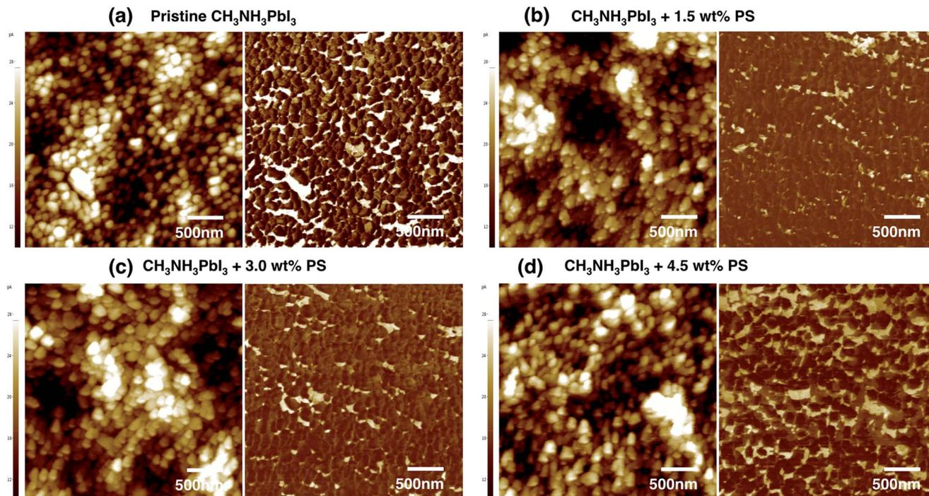
Fig. 3 Surface properties of thin films used in this work. The (a–d left panels) atomic force microscopy (AFM) and (a–d right panels) conductive AFM (cAFM) images of  $\text{CH}_3\text{NH}_3\text{PbI}_3$  perovskite thin film with different concentrations of polystyrene on the ITO/PEDOT:PSS layer.
