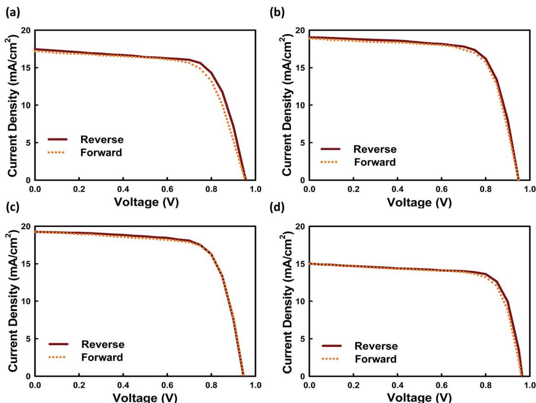
Fig. 7  $J$ - $V$  plots for perovskite solar cells (a) without PS, (b) with 1.5 wt% PS, (c) with 3.0 wt% PS, and (d) with 4.5 wt% PS under one sun conditions (100 mW cm<sup>-2</sup>, AM1.5G). The scan rate for both scans is 10 mV s<sup>-1</sup>.
