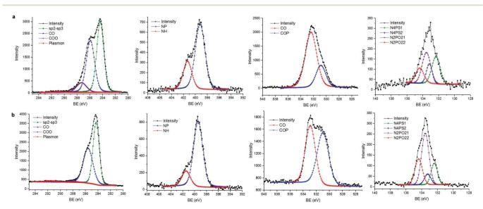
XPS analyses (from left to right: binding energy of carbon, nitrogen oxygen and phosphorus elements) of (a)  $DG_4$ -GO and (b)  $DG_4$ -RGO.
