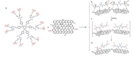
Scheme 1 Chemical interplay occurring at the dendrimer–graphene oxide interface. (a) Typical chemical structure of the first generation phosphorus dendrimer  $DG_1$  and oxygenated graphene oxide sheets. (b) Plausible mechanism occurring during interfacial complexation of ternary diethyl-N-amino-ammonium chloride arms and (c and d) the subsequent chemical reduction. See S10 in the ESI† for further discussion.
