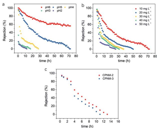
Fig. 8 Continuous filtration operation: (a) rejection rates of the CPNM-1 to Pb(II) aqueous solution under different pH environments (pH = 2–6;  $C_0 = 10 \text{ mg L}^{-1}$ ; 25 °C); (b) rejection rates of the CPNM-1 to Pb(II) aqueous solution with different initial concentrations (pH = 5;  $C_0 = 10\text{--}50 \text{ mg L}^{-1}$ ; 25 °C); (c) changes of rejection ratio of the CPNM-2 and CPNM-3 to Pb(II) aqueous solution with filtration time (pH = 5;  $C_0 = 10 \text{ mg L}^{-1}$ ; 25 °C).
