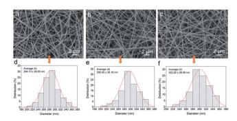
Fig. 1 SEM images of the nanofibers with different mass ratios of CA and PMAA: (a) CPNM-1, (b) CPNM-2, and (c) CPNM-3; (d), (e) and (f) are their corresponding diameter distribution.
