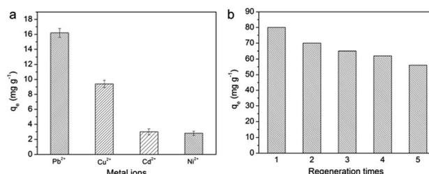
Fig. 7 (a) Pb(II) competitive uptake in a mixed bivalent metal ion solution (pH = 6;  $V = 30$  mL;  $m$  [adsorbent] = 30 mg;  $C_0$  [Pb(II)] = 25  $\text{mg L}^{-1}$ ; 25 °C); (b) regeneration times of the adsorption process for Pb(II) removal by CPNM-1 (pH = 6;  $V = 30$  mL;  $m$  [adsorbent] = 30 mg;  $C_0$  [Pb(II)] = 100  $\text{mg L}^{-1}$ ; 25 °C).
