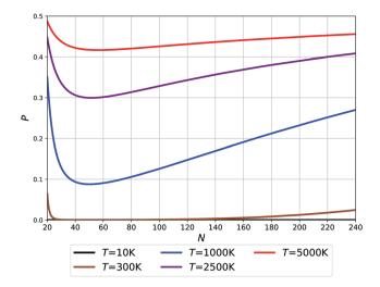
Fig. 5 Probability of O clusters (relative to F) as a function of size at 10 K, 300 K, 1000 K, 2500 K, and 5000 K temperatures
