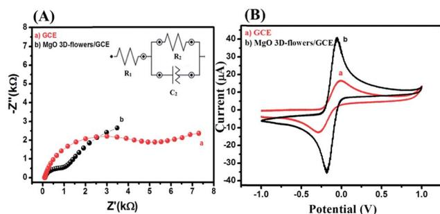
Fig. 4 Nyquist plots (A) and CVs (B) of the bare GCE (a) and MgO 3D-flowers/GCE sensor (b) in the presence of 5 mM  $K_3 [Fe(CN)_6] / K_4 [Fe(CN)_6]$  in 0.1 M PBS (pH = 7.0). Inset: equivalent circuit.
