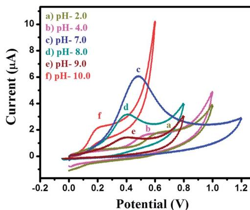
Fig. 6 Cyclic voltammograms of the MgO 3D-flowers/GCE sensor in the presence of 25  $\mu\text{M}$  4-CP in 0.1 M PBS at different pH (2, 4, 7, 8, 9 and 10) with a scan potential of 100  $\text{mV s}^{-1}$ .
