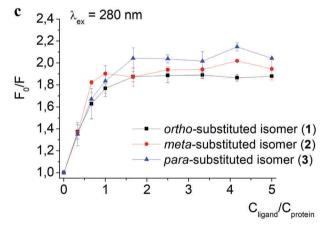
Fig. 2 Stern-Volmer plots of fluorescence intensity quenching of BSA emission excited at 280 (a) and 295 (b) nm, as well as of HSA emission excited at 280 nm (c), by clathrochelates 1-3;  $F_0$  and F are protein fluorescence intensities in the absence and in the presence of these complexes. Spectra were recorded in 0.05 M Tris HCl, pH 7.9
