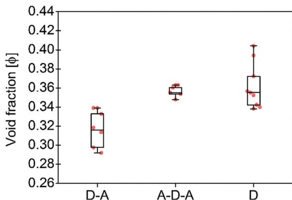
**Fig. 3** Calculated void fractions  $\phi$  for the three family molecules studied in this work and listed in Table 1. The box plot denotes median (centre line), 25th quartile (bottom edge of the box), 75th quartile (top edge of the box), maximum and minimum values. Only non-solvated structures have been considered.
