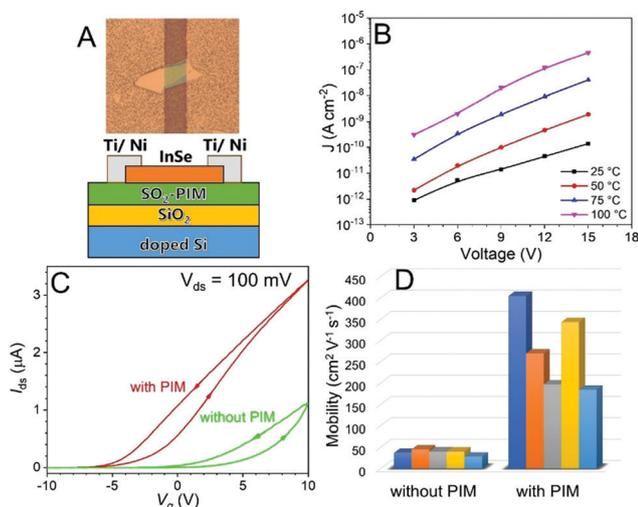
Fig. 4 (A) Schematic of the InSe-based FET device and the top-view optical microscopy image. (B) Leakage current density as a function of voltage in a capacitor device. (C) The  $I_{\text{ds}}-V_{\text{g}}$  transfer curve and (D) comparison of electron mobility in InSe for the FET devices with and without  $\text{SO}_2$ -PIM. Five devices were tested for each type of FET.
