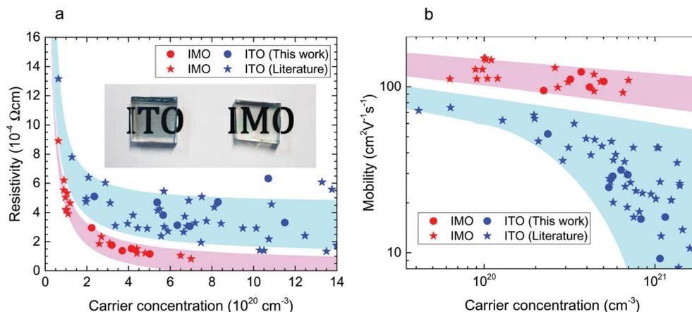
**Fig. 2** Transport properties. (a) Resistivity versus free carrier concentration for polycrystalline ITO and IMO films. Inset shows a photograph of ITO and IMO films. (b) Hall mobility versus free carrier concentration. Data from this work are circles. Data plotted as stars are taken from the literature for IMO<sup>11–16</sup> and ITO<sup>12,17–22</sup> films. In this carrier concentration regime, the electron mobility is limited by ionized impurity scattering.
