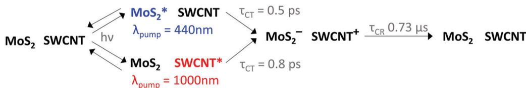
Fig. 5 Kinetic scheme highlighting the different time constants for hole transfer ( $\tau_{HT}$ ) versus electron transfer ( $\tau_{ET}$ ) resulting from either selective MoS<sub>2</sub> or SWCNT excitation using pump wavelengths ( $\lambda_{\text{pump}}$ ) of 440 and 1000 nm, as well as the time constant for charge recombination ( $\tau_{CR}$ ) from the amplitude-averaged lifetime of a triexponential fit.
