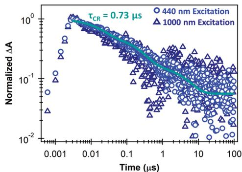
Fig. 3 Carrier kinetics at 1175 nm (trion induced absorption) on the microsecond time scale for monolayer MoS<sub>2</sub>/SWCNT heterojunctions under 440 nm excitation (light blue circles) or 1000 nm excitation (dark blue triangles), showing a triexponential fit with an amplitude-averaged charge recombination time constant ( $\tau_{CR}$ ) of 0.73  $\mu$ s.
