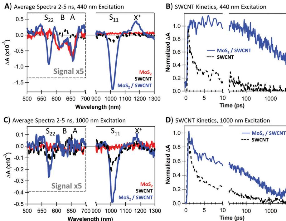
Fig. 2 (A) Transient absorption spectra averaged over 2–5 ns following 440 nm excitation of neat MoS<sub>2</sub> (red), neat SWCNT (black dotted), and MoS<sub>2</sub>/SWCNT heterojunctions (blue); (B) kinetic traces at 1175 nm, corresponding to the SWCNT trion (X<sup>+</sup>) induced absorption with 440 nm excitation; (C) transient absorption spectra averaged over 2–5 ns following 1000 nm excitation; (D) kinetic traces at the SWCNT trion induced absorption with 1000 nm excitation.
