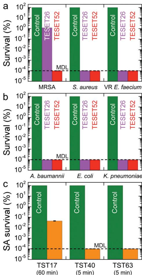
Fig. 2 Survival of (a) Gram-positive and (b) Gram-negative bacteria after exposure to a control (green), TESET26 (purple) and TESET52 (red) for 5 min. In (c), the survival of methicillin-susceptible *S. aureus* is presented for three TST polymers varying in midblock sulfonation content (exposure times are included).
