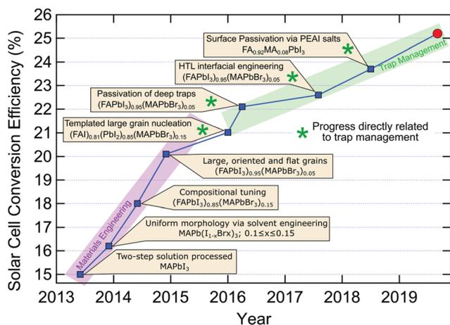
Fig. 5 Overview of recent progress in single junction perovskite solar cell efficiency, identifying the key technological advances.<sup>59–61,75,80,120,134,137,138</sup> The red circle indicates the current record (25.2%) confirmed by National Renewable Energy Laboratory (NREL).<sup>139</sup>
