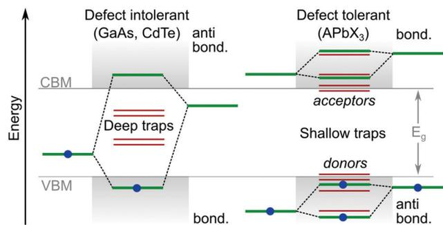
Fig. 4 Comparison of typical trap energies relative to the electronic band structure of traditional defect intolerant compound semiconductors (*i.e.* III–V and II–VI varieties) and defect tolerant<sup>43</sup> lead halide perovskite materials.<sup>1,2</sup>
