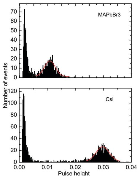
Fig. 4 Pulse height spectra of scintillators excited through  $\alpha$ -particle interaction from <sup>241</sup>Am in MAPbBr<sub>3</sub> at 50 K and CsI at 50 K before correction for the spectral response of the photomultiplier. The pulse height distributions that signify scintillation response due to  $\alpha$ -particles are fitted by Gaussians (red lines).
