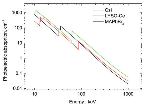
**Fig. 6** Photoelectric fractions of absorption of gamma-rays in CsI, LYSO-Ce and MAPbBr<sub>3</sub>. The data are calculated using an XCOM web-tool.<sup>50</sup>
