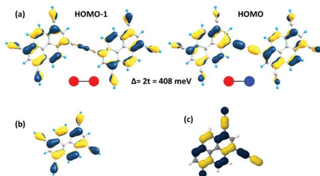
Fig. 3 (a) Illustration of the HOMO–1 and HOMO wavefunctions in the Pyr-COF dimer and estimation of the transfer integrals ( $t$ ) for holes, based on the energy-splitting approach;  $\Delta$  denotes the difference between the HOMO and HOMO–1 energies of the dimer; the red and blue dots express the symmetry of the tight-binding wavefunctions. (b) HOMO of the pyrene building block. (c) Wave-function of the valence band maximum of the 2D Pyr-COF at the  $\Gamma$ -point.
