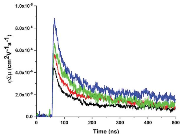
Fig. 5 Representative fp-TRMC transients with increasing fluence ( $1 \times 10^{14}$ – $4 \times 10^{15}$  photons per  $\text{cm}^2$ ) for a ZnPor-COF-PS film at 700 nm photoexcitation with 7 ns pulse width.
