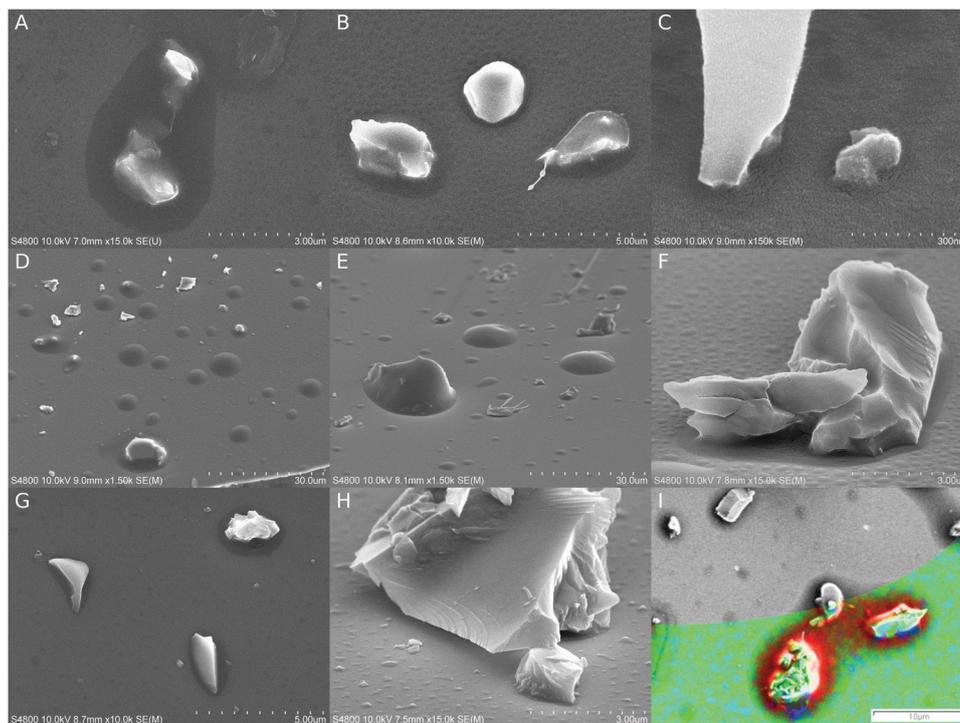
**Fig. 3** FESEM micrographs of glass substrates. (A–C) 8 min initiation at 95%, 50% and 18% SRs, respectively. (D–F) 15 min initiation at >95%, 50% and 18% SRs, respectively. (G and H) 15 min initiation with added oxygen at 95% and 50% SRs, respectively. (I) Composite image combining an FESEM micrograph (grayscale) and an EDS element map (color). Red: C, green: O, and blue: Si. 15 min UV irradiation at >95% SR, N<sub>2</sub> as the carrier gas.
