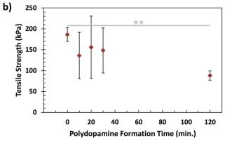
Fig. 4 Effects on final underwater adhesive tensile strength of (a) water content of dopamine-Fe3+-Tris (D-Fe-Tris) solution (effectively diluting or concentrating these three components before application) and (b) polydopamine formation time before application. In both plots, \* refers to a p-value < 0.05, while \*\* refers to a p-value < 0.01, each between the pair of conditions
