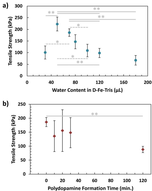
Fig. 4 Effects on final underwater adhesive tensile strength of (a) water content of dopamine– $\text{Fe}^{3+}$ –Tris (D–Fe–Tris) solution (effectively diluting or concentrating these three components before application) and (b) polydopamine formation time before application. In both plots, \* refers to a  $p$ -value  $< 0.05$ , while \*\* refers to a  $p$ -value  $< 0.01$ , each between the pair of conditions.
