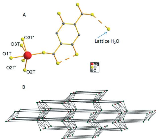
Fig. 1 A. Representation of the structure of complex **1** with labelling of the terminal water O atoms. The dashed lines indicate H-bonding interactions. Hydrogen atoms were omitted for clarity. B. The real (4,12)-coordinated hydrogen bonded 3D network in **1**. Color code: 12-c nodes green, 4-c nodes red.
