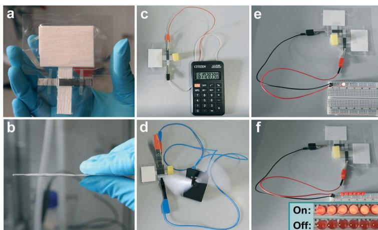
Fig. 6 A paper-based  $\mu\text{Al}$ -air pouch battery from (a) top and (b) side view. (c) A single battery (geometric electrode active area:  $8 \times 5 \text{ mm}^2$ ) powering a calculator. (d) A single battery (geometric electrode active area:  $8 \times 15 \text{ mm}^2$ ) powering a mini-fan. Two series-connected  $\mu\text{Al}$ -air pouch batteries (geometric electrode active area:  $8 \times 5 \text{ mm}^2$ ), powering (e) one and (f) six LED lamp(s).
