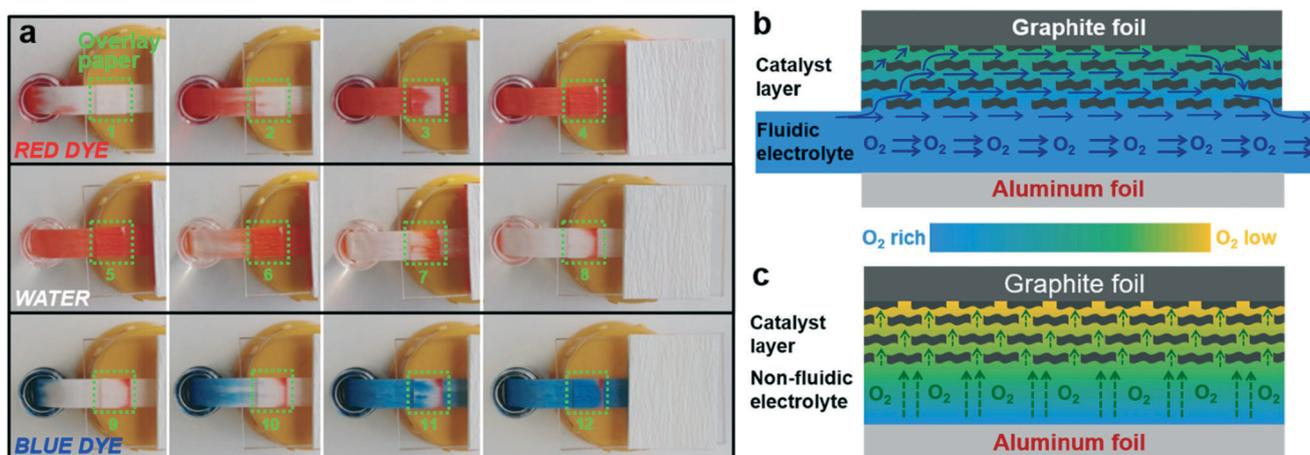
Fig. 4 (a) Time-lapse photos showing flow patterns of solutions within the overlay paper, where the green squares mark the overlay paper. Schematic illustrations of  $O_2$ -rich/low electrolyte distribution in (b)  $\mu$ Al-air battery, and (c) non-fluidic Al-air battery in cross-section.
