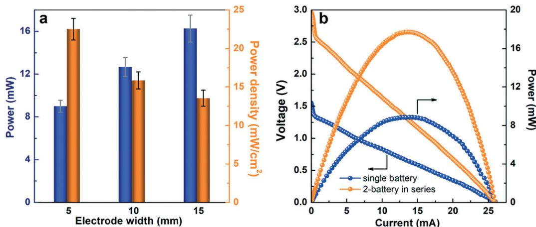
Fig. 5 (a) Comparison of power/power density in paper-based  $\mu\text{Al}$ -air batteries with three electrode sizes (geometric electrode active area:  $8 \times 5$ ,  $8 \times 10$ ,  $8 \times 15 \text{ mm}^2$ ). (b) Polarization ( $V-I$ ) and power density curves of a single battery and two paper-based  $\mu\text{Al}$ -air batteries connected in a series.
