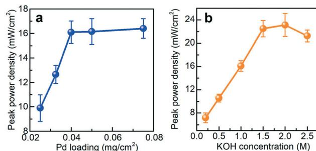
Fig. 2 (a) Influence of the Pd loading on peak power density. KOH concentration: 1.0 M; the geometric electrode active area:  $8 \times 5 \text{ mm}^2$ . (b) Influence of the KOH concentration on the peak power density. Pd loading: 0.04  $\text{mg cm}^{-2}$ ; the geometric electrode active area:  $8 \times 5 \text{ mm}^2$ .
