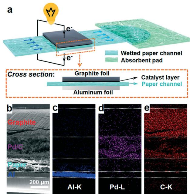
Fig. 1 (a) Schematic illustration of a paper-based  $\mu$ Al–air battery; (b) cross sectional SEM image; and (c–e) EDS elemental mapping images of a paper-based  $\mu$ Al–air battery.
