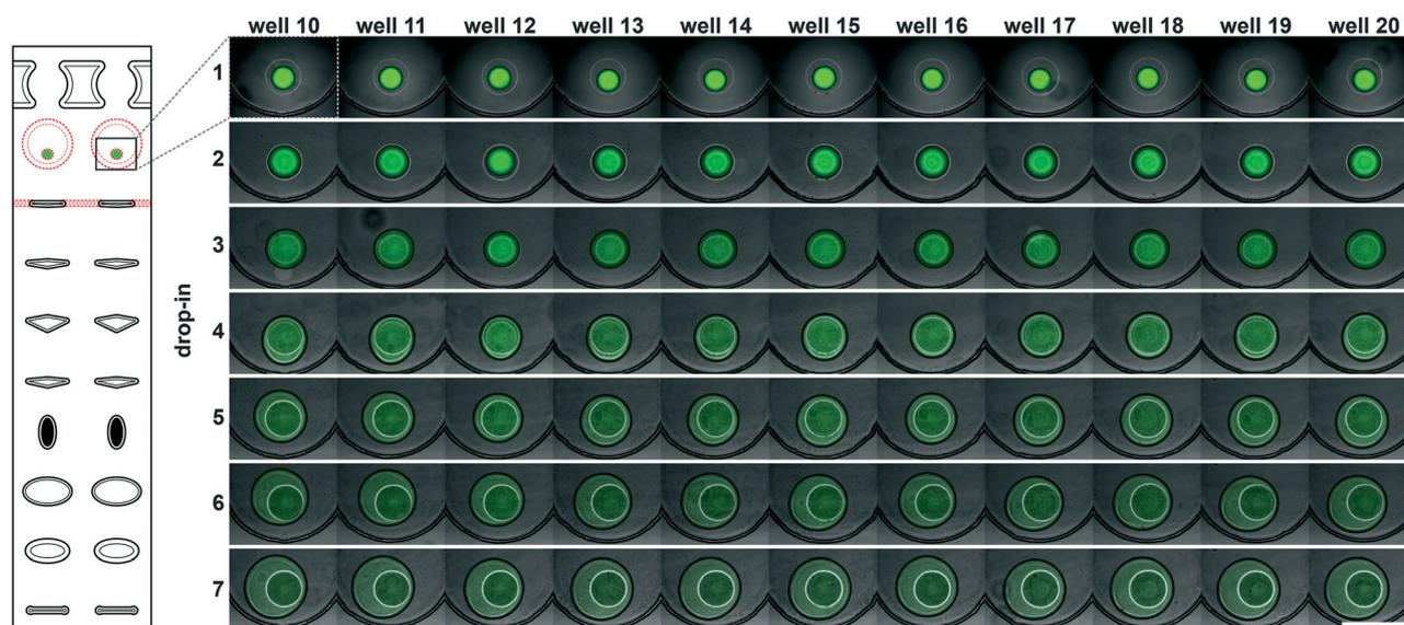
Fig. 3 A subset of the multistep SlipChip device (wells 10–20) showing overlaid fluorescence and bright-field images after each of seven drop-in and merging events of 3 nL 50  $\mu\text{M}$  Alexa Fluor 488 droplets. Scale bar: 500  $\mu\text{m}$ .
