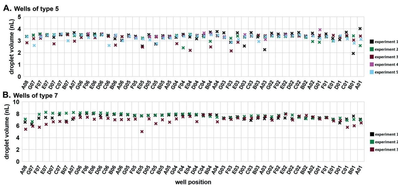
Fig. 4 Reproducibility and spatial distribution of volume metering by carrier wells in the multistep SlipChip. (A) Wells of type 5, measured volumes of  $3.30 \pm 0.31$  nL (mean  $\pm$  S.D.); (B) wells of type 7 measured volumes of  $7.36 \pm 0.57$  nL (mean  $\pm$  S.D.).
