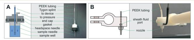
Fig. 3 (A) Diagram and corresponding image of the dual-lumen 'sipper' needle. A rubber gasket seals the needle assembly against a multiwell plate, allowing air pressure applied to the headspace to drive fluid into the sample needle and subsequently onto the device. (B) Diagram and image of the sheath nozzle, which cleanses the tubing outlet after sample collection with a coaxial sheath fluid (e.g. air, water, or oil).
