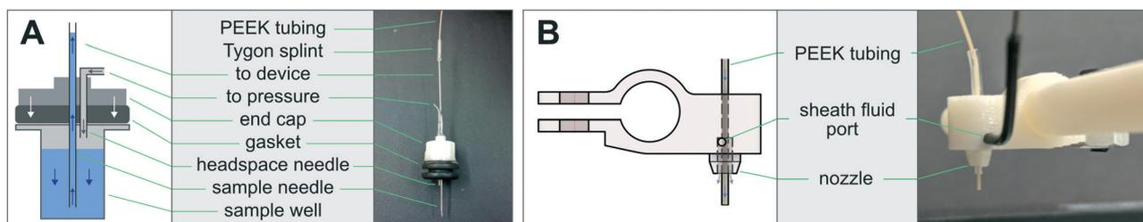
**Fig. 3** (A) Diagram and corresponding image of the dual-lumen 'sipper' needle. A rubber gasket seals the needle assembly against a multiwell plate, allowing air pressure applied to the headspace to drive fluid into the sample needle and subsequently onto the device. (B) Diagram and image of the sheath nozzle, which cleanses the tubing outlet after sample collection with a coaxial sheath fluid (e.g. air, water, or oil).
