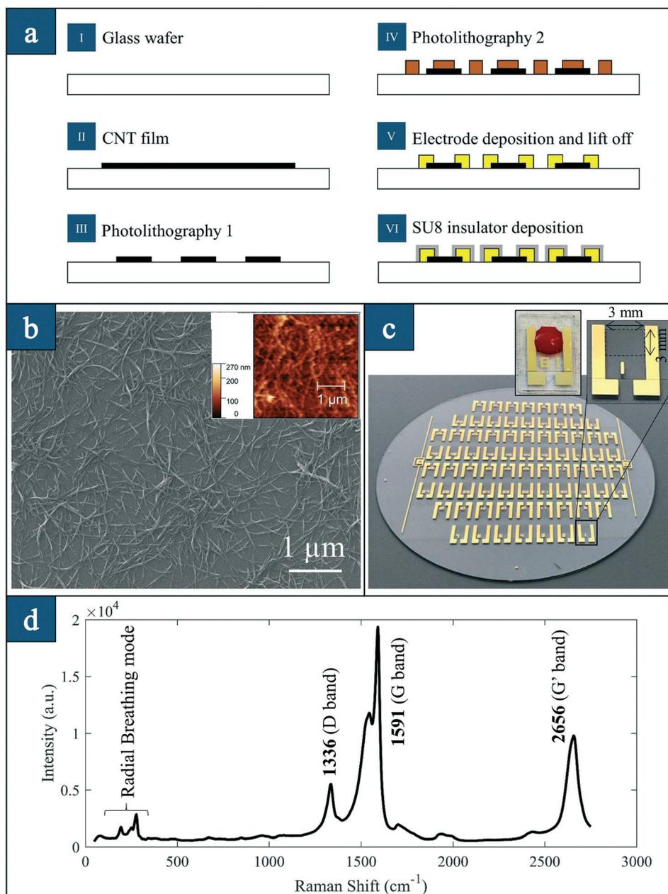
**Fig. 2** Device fabrication and characterization: (a) flowchart of device fabrication; (b) scanning electron micrograph (SEM) of nanotubes; the inset is an atomic force microscopy (AFM) image of a nanotube film; (c) optical image of an entire wafer consisting of a 76-element array; the inset is the individual devices (blank and blood adsorbed); (d) Raman spectroscopy of carbon nanotubes; a small D band, large G band and pronounced 2D band suggest the carbon nanotube structure.
