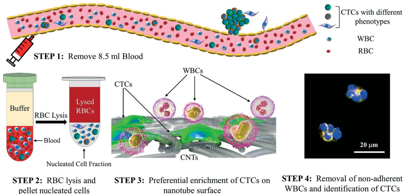
Fig. 1 The nanotube-CTC-chip: steps in isolation and enumeration of CTCs using the nanotube-CTC-chip.
