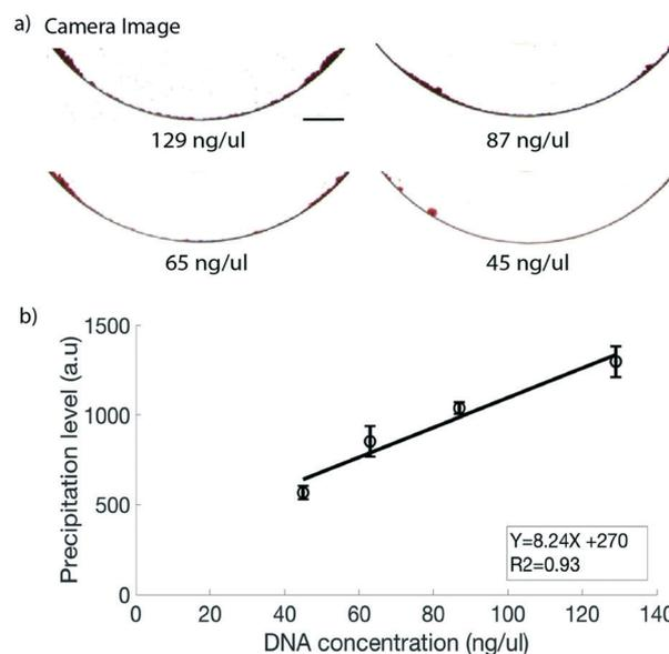
**Fig. 4** DNA quantification on the LOD platform. CMOS sensor generated precipitate images of a known amount of PCR product. a) Four different concentrations imaged with a CMOS camera with  $45 \text{ ng } \mu\text{l}^{-1}$  being the lowest detectable concentration. Scale bar: 1 mm. b) Calibration curve of the precipitation level versus known DNA concentration.
