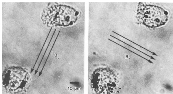
**Fig. 7** Study of mechanical properties of cells using rotating MPs. Shown are two lung macrophages, from experiments by Valberg *et al.* in 1987.<sup>47</sup> The dark spots are aggregates of magnetic nanoparticles. The direction of the applied field is indicated with the arrows. Small arrow heads indicate the reorientation of the magnetic aggregates.
