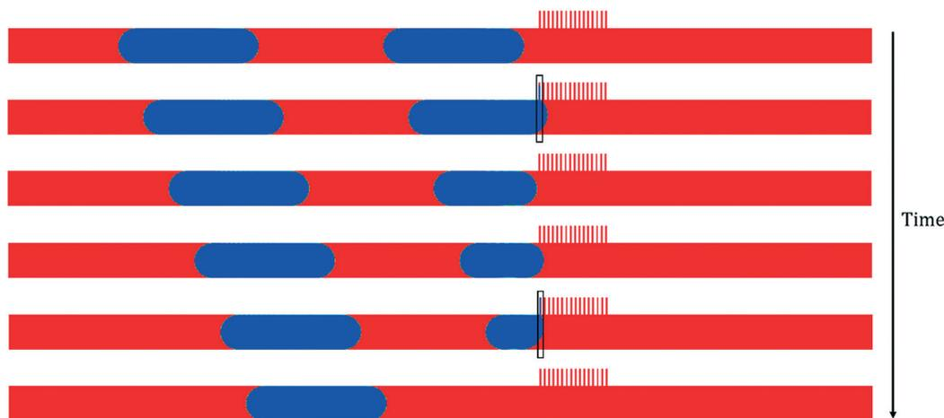
Fig. 4 Time-lapse snapshots of the phase distribution in a capillary microseparator during breakthrough ( $\Delta P_{\text{outlet}} = 3640$  Pa). Here, toluene is the wetting phase (red) and water is the non-wetting phase (blue).  $\Delta t = 0.05$  s. The black box highlights the capillaries through which breakthrough occurred.
