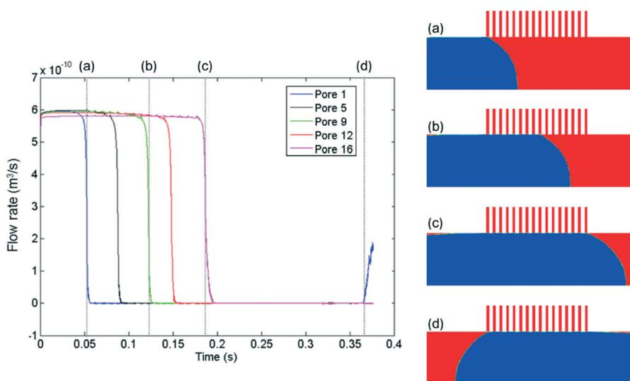
**Fig. 6** Real-time flow rates through different capillary pores obtained from CFD simulation. In this case, a segment of non-wetting phase moved through the capillary region without entering into the pores, corresponding to the normal operation regime. Pore 1 referred to the leftmost capillary channel, while pore 16 was the rightmost. Only the top half of the channel was simulated (with symmetric boundary condition on the bottom) to reduce computation time.
