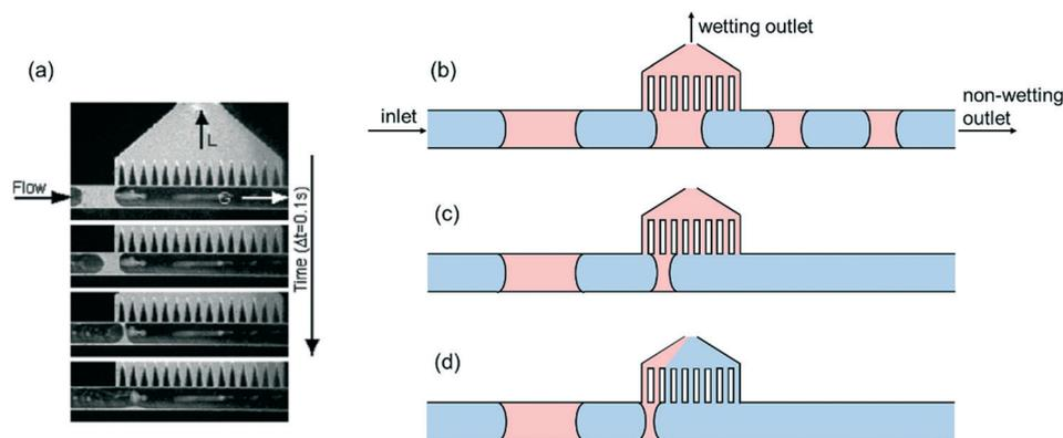
Fig. 1 (a) A series of photographs demonstrating the separation of a gas/liquid mixture using the capillary separator<sup>22</sup> (copyright 2005 by American Chemical Society); scheme of the different operation modes of the capillary separator when varying the pressure difference between the non-wetting and wetting outlets: (b) retention; (c) complete separation; (d) breakthrough.
