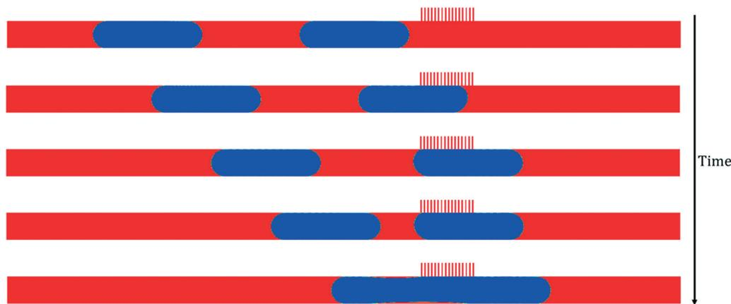
Fig. 3 Time-lapse snapshots of the phase distribution in a capillary microseparator during normal operation ( $\Delta P_{\text{outlet}} = 1820$  Pa). Here, toluene is the wetting phase (red) and water is the non-wetting phase (blue).  $\Delta t = 0.15$  s.
