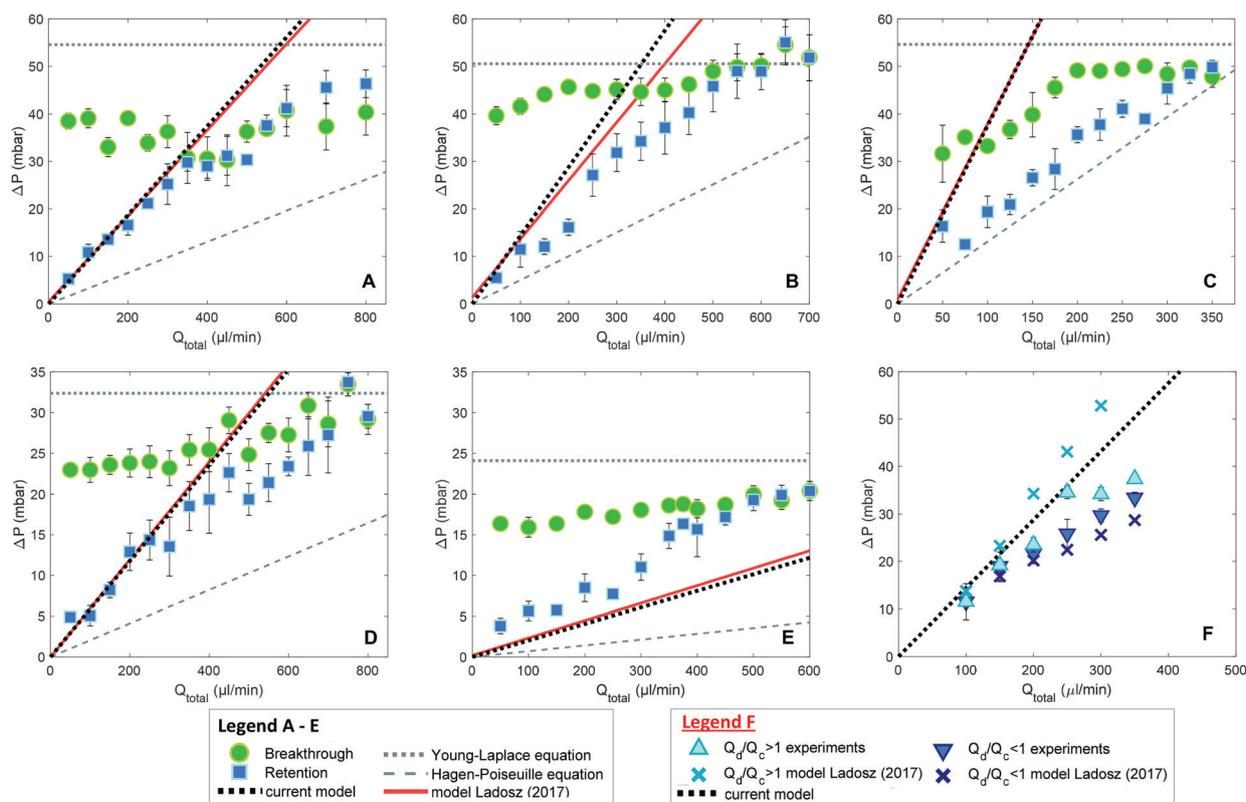
**Fig. 8** Comparison of model predictions in this work with the results of Ładosz and Rudolf von Rohr;<sup>48</sup> A–F: flow rate ratio equal to one, five capillary geometries were tested, with capillary dimensions denoted in  $\mu\text{m}$  as width-length: A: 10–250; B: 10–500; C: 10–1000; D: 20–1000; E: 30–1000; F: varied flow rate ratio experiments using separator 10–500, only retention bound shown.
