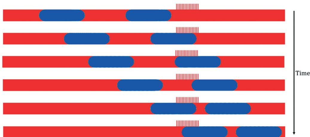
Fig. 5 Liquid-liquid phase distribution in a capillary microseparator capturing the retention phenomenon ( $\Delta P_{\text{outlet}} = 30$  Pa). Here, toluene is the wetting phase (red) and water is the non-wetting phase (blue).  $\Delta t = 0.15$  s.
