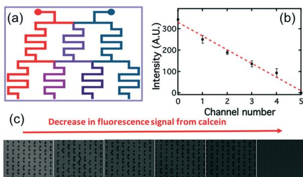
**Fig. 4** (a) Schematic showing the principle of the “tree shape network” design that generates a linear concentration gradient. (b) Measurements of the concentration gradient of calcein formed in the six trap chambers, at a flow rate of  $0.2 \mu\text{L min}^{-1}$ , measured by determining the fluorescence intensity of the calcein. The behavior can be described by the linear fit shown in red. (c) Fluorescence images taken for different trap chambers.
