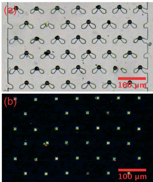
Fig. 6 Images of the PC/PG coated E7 droplets trapped in the swallowtail shaped trap structures in one of the chambers. (a) Bright field image; (b) image taken using polarized microscopy in transmission.
