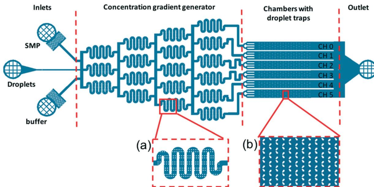
**Fig. 3** Trap structure with a concentration gradient generator used to evaluate the Smp43 detection by the lipid-coated LC droplets. The device has four main parts: inlets, concentration gradient generator, chamber with droplet traps, and outlet. (a) Expanded view of the serpentine channel and pillars in the channel to promote mixing; (b) expanded view of the trap region indicating how the droplets are trapped in the swallowtail features.
