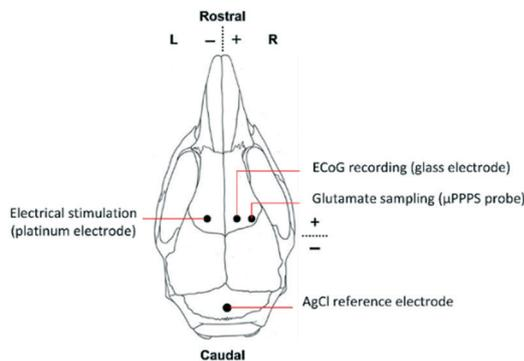
Fig. 4 Schematic representation of a mouse skull indicating locations of the  $\mu$ PPPS probe in relation to the stimulation site, ECoG and reference electrode during *in vivo* experiments in an anesthetized mouse.
