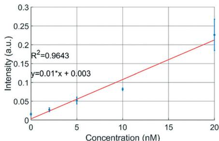
Fig. 6 Fluorescence measurements with resorufin sodium salt demonstrate that concentrations  $< 2 \text{ nM}$  can be measured using the developed optical detection setup (see text for details). Resorufin was injected directly into the optical detection capillary ( $n = 3$ ).
