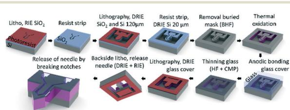
**Fig. 3** Schematic overview of the fabrication process of the  $\mu$ PPPS probe. Note that the probe and layer thicknesses are not drawn to scale. See text for a full description, and Table S6† for a more detailed process flow.
