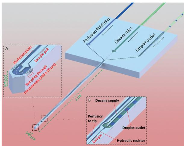
**Fig. 1** Schematic visualization of the  $\mu$ PPPS principle. Sample from tissue is collected through small sampling channels (see sampling tip inset, A). A push-pull configuration inside the needle ensures rapid transport of the sample to the external measurement equipment. A droplet generator is either integrated in the shaft of the probe (see droplet generator inset, B; probe type 1) or located externally (probe type 2), to prevent dispersion and to maintain a good temporal resolution.
