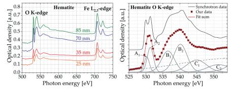
Fig. 6 (Left) Oxygen K-edge and iron  $L_{2,3}$ -edge spectra of hematite samples of different thickness (accumulated over 1000 pulses). (Right) NEXAFS spectrum of hematite sample (thickness 35 nm) at the oxygen K-edge fitted with 6 Gaussian peaks (thin solid lines) and one arctan function (thin dashed line) in comparison to synchrotron data.<sup>33</sup> The samples have been provided by the group of F. de Groot (University of Utrecht, Netherlands).
