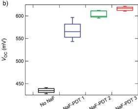
Fig. 5 (a) Molar fraction of Na of four different samples with different amounts of Na incorporated derived from GD-OES measurements. (b) Open-circuit voltage of the corresponding solar cells.
