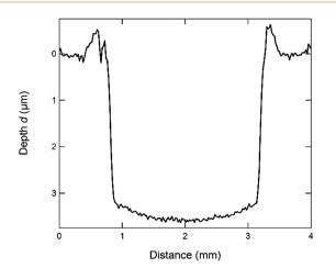
Fig. 1 Profilometer scan of a sputtered crater in a Mo/CIGSe layer stack. The image shows an average of 21 line scans taken within a distance of  $\sim$ 0.4 mm in the middle of the file; moderate voltage and pressure were chosen in the present study.
