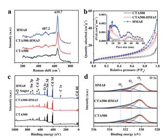
Fig. 3 (a) Raman spectra. (b) BET surface area measurement of the  $Cd_2SnO_4$  photoanodes and pore size distribution (inset) of the  $Cd_2SnO_4$  photoanodes. (c) Survey scan XPS spectra of CTA500, CTA500-HMA5 and HMA8, respectively. (d) O 1 s XPS spectra of typical CTA500, CTA500-HMA5 and HMA8 samples.
