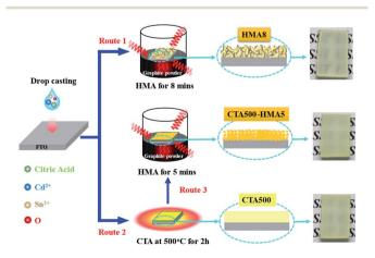
Fig. 1 Schematic representation for preparation of Cd<sub>2</sub>SnO<sub>4</sub> thin films
