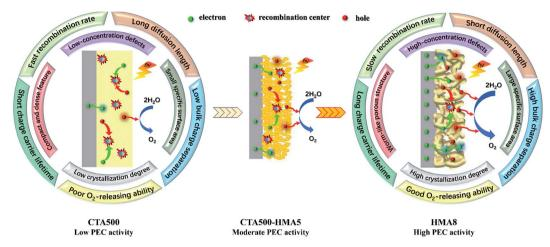
Fig. 7 Proposed photoelectrocatalytic mechanisms for CTA500, CTA500-HMA5 and HMA8 photoanodes.
