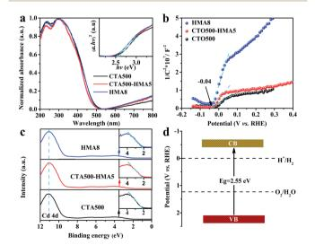
Fig. 4 (a) UV-Vis absorption spectra and the Tauc plots (inset) of the CTA500, CTA500-HMA5 and HMA8 samples. (b) Estimation of  $E_{\rm FB}$  using MS plots. (c) Estimation of the VBM by valence-band XPS spectroscopy. (d) The proposed energy band structure of deficient Cd<sub>2</sub>SnO<sub>4</sub> determined using Tauc plots, MS plots and valence-band XPS spectroscopy.
