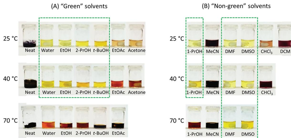
**Fig. 1** Stability evaluation of HMF in various solvents. According to the CHEM21 recommendation, the 12 tested solvents were categorized as "Green" and "Non-green".<sup>54</sup> Neat condition (solvent-free) was categorized as "Green". The photos were taken after the solutions of HMF had been stirred for 5 h with *p*-TsOH at 25, 40, and 70 °C. The solutions without significant HMF degradation (coloration) are highlighted by green dashed boxes.
