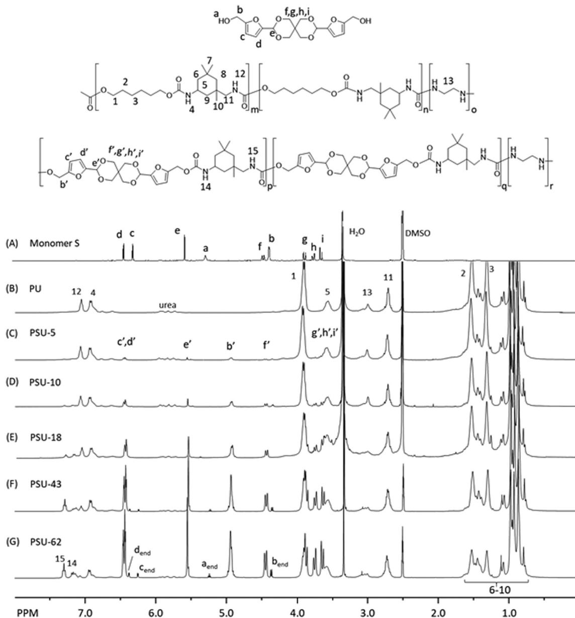
Fig. 7  $^1\text{H}$  NMR spectra of (A) Monomer S and (B–G) poly(urethane-urea)s.
