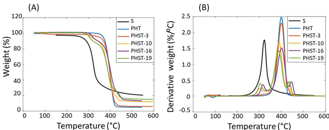
Fig. 5 (A) TGA thermograms and (B) first derivative curves of Monomer **S** and the polyesters.
