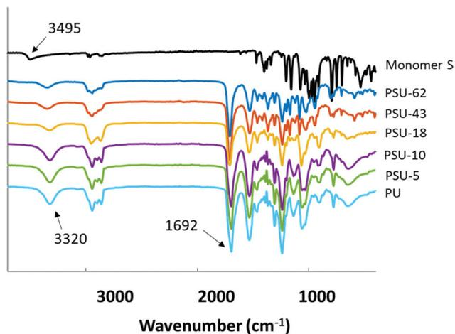
Fig. 8 FTIR-spectra of Monomer S and poly(urethane-ureas).
