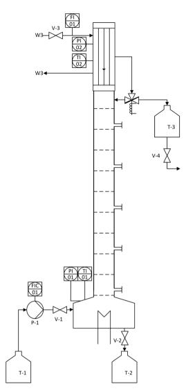
Fig. 6 Schematic depiction of the rectification setup used for the reactive distillation of the MeOH/FA/1,2-DMI mixture.
