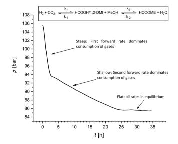
Fig. 4 Pressure/time profile for the hydrogenation of  $CO_2$  under prolonged reaction time (conditions see Table 2; additional  $6^{th}$  cycle using an amine concentration of  $c_{1,2-\mathrm{DMI}} = 2.3 \, \mathrm{mol} \, \mathrm{L}^{-1}$ ).
