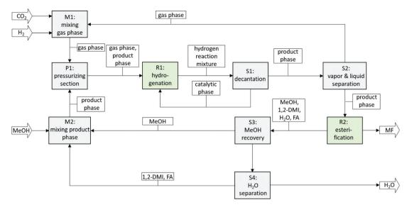
Fig. 8 Block flow diagram of a continuous process for the production of MF from CO<sub>2</sub>. Ri = Reaction units, Si = separation units, Mi = mixing units.
