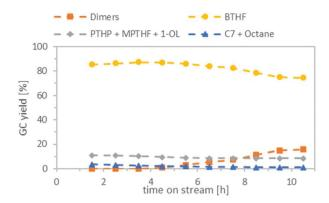
Fig. 8 Continuous flow hydrogenation and deoxygenation of a FFA solution (0.25 mol  $L^{-1}$ ) in cyclohexane. Conditions: Catalyst bed  $1^{\rm st}$  reactor: 1 g Ru/C, 50 °C, WHSV = 2 h<sup>-1</sup>, catalyst bed  $2^{\rm nd}$  reactor: 1 g Ru/C + 6 g Amberlyst 36, 150 °C, WHSV = 0.29 h<sup>-1</sup>, substrate flowrate: 1 mL min<sup>-1</sup>, hydrogen flowrate: 50 mL<sub>N</sub> min<sup>-1</sup>, pressure: 80 bar. C7 = n-heptane and 2-methyl-5-ethyltetrahydrofuran.
