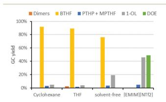
Fig. 5 Influence of the solvent on the deoxygenation of THFA. Conditions: THFA (0.75 mmol), Ru/C (3.75  $\mu$ mol Ru), Amberlyst-36 (9.3 mg, 0.05 mmol H<sup>+</sup>), H<sub>2</sub> (80 bar), 150 °C, 6 h, solvent (1.5 mL). [Emim][NTf2] = 1-ethyl-3-methylimidazolium bis(trifluoromethyl-sulfonyl)imide.
