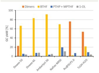
Fig. 4 Comparison of different acid components for the deoxygenation of THFA. Conditions: THFA (0.75 mmol), Ru/C (3.75  $\mu$ mol Rul), H $^+$  (0.05 mmol), H $_2$  (80 bar), 150 °C, cyclohexane (1.5 mL), 6 h.
