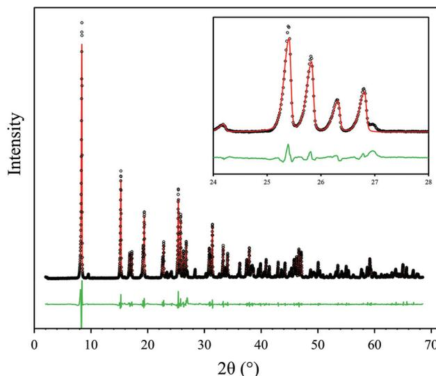
**Fig. 2** PXRD pattern of MFM-300(Al)-MW. Black = observed; red = simulated pattern Le Bail fit; green = difference plot. Inset: Plot of the PXRD pattern between 24 and 28° 2θ; an extra reflection attributed to unreacted linker is visible at ~27° 2θ in the difference plot.
