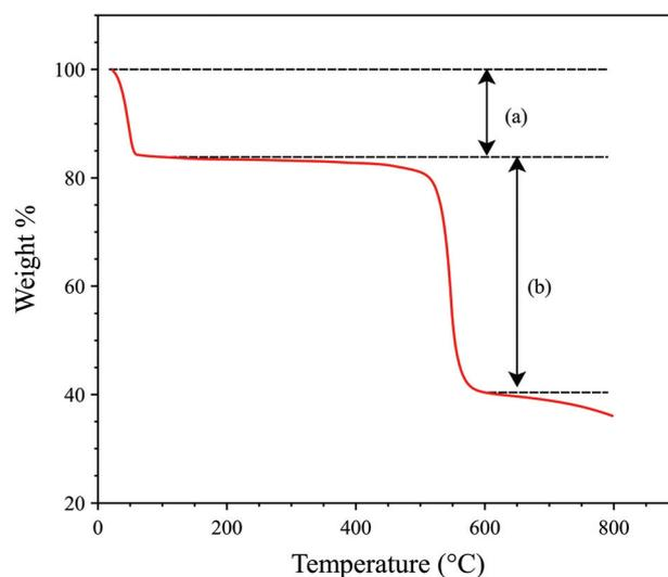
**Fig. 3** TGA thermogram of MFM-300(Al)-MW. (a) 30–100 °C = loss of adsorbed water (15.85%) from the MOF. (b) 465–600 °C = thermal decomposition of MFM-300(Al)-MW (40.23%). Slow MOF decomposition is observed beyond 600 °C.
