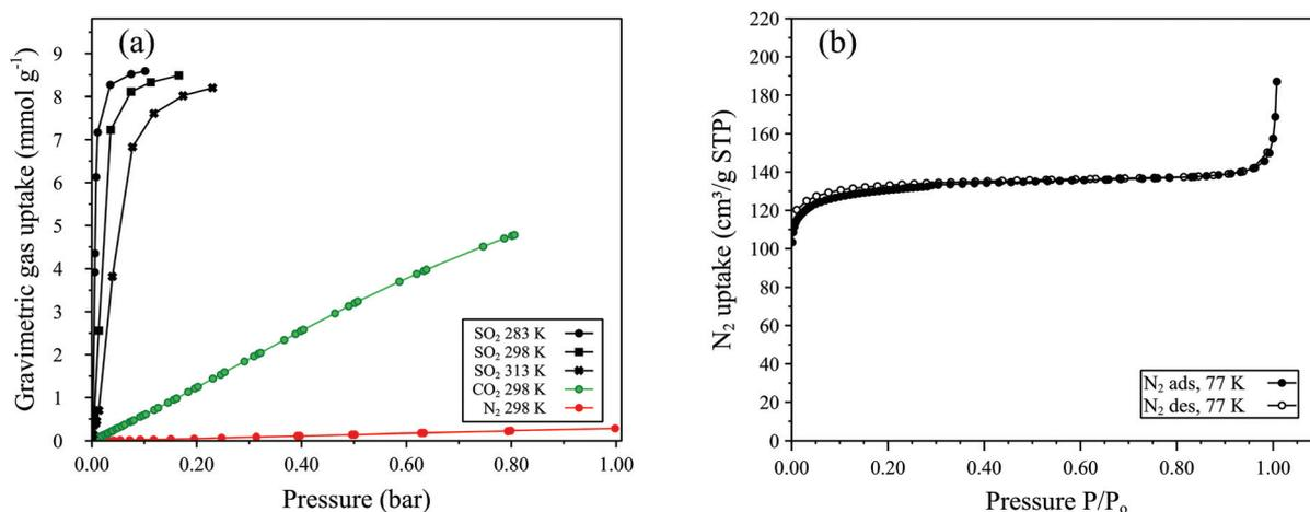
Fig. 5 (a) Gravimetric SO<sub>2</sub> and manometric CO<sub>2</sub>, and N<sub>2</sub> gas adsorption isotherms and (b) manometric N<sub>2</sub> gas sorption isotherm at 77 K for MFM-300(Al)-MW. Legends inset. SO<sub>2</sub> data were collected using 25% SO<sub>2</sub> in N<sub>2</sub> as the sorbate.
