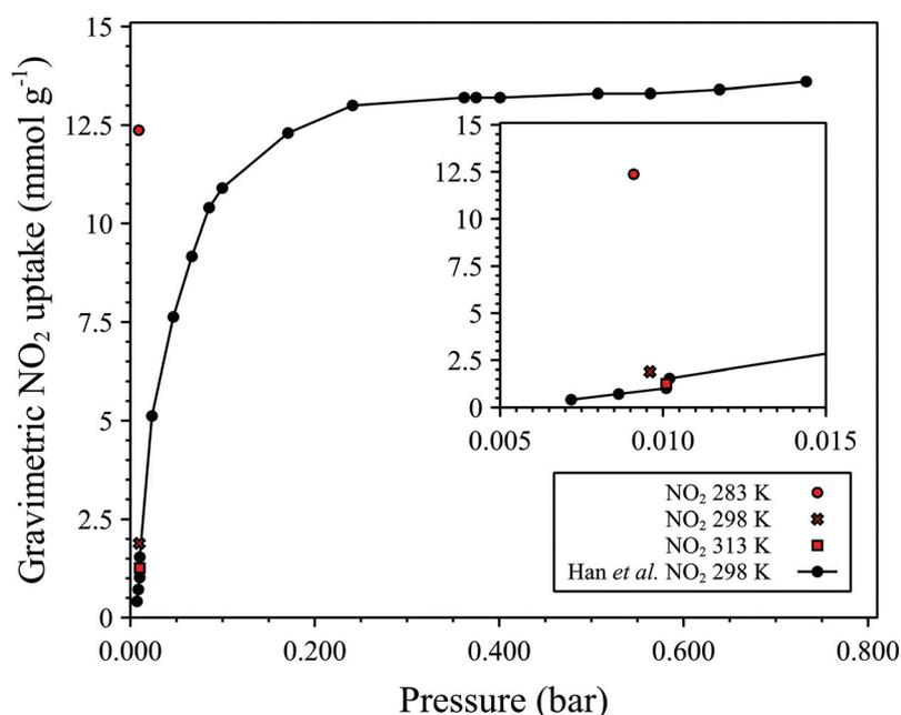
**Fig. 6** Single point NO<sub>2</sub> sorption data collected for MFM-300(Al)-MW at 283 K, 298 K, and 313 K corresponding to partial pressures between 0.009 and 0.01 bar using 1% NO<sub>2</sub> in N<sub>2</sub> as the sorbate (in red). NO<sub>2</sub> isotherm at 298 K reported by Han *et al.* (ref. 10) for MFM-300(Al)-CH for comparison in black (sorbate is pure NO<sub>2</sub>). Legend inset.
