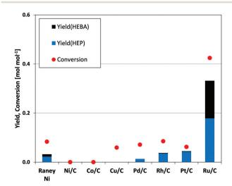
Fig. 4 Screening of catalytic metals for N-(2-hydroxyethyl)succinimide hydrogenation. (Cond.: 150 °C, 150 bar H<sub>2</sub>, 6 h, 750 rpm, 37.5 mg catalyst).
