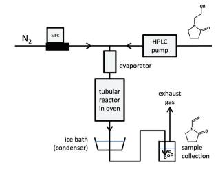
Fig. 7 Simplified schematic of the gas phase dehydration of N-(2-hydroxyethyl)pyrrolidones in lab-scale. Vinylpyrrolidone monomers are obtained after condensing the product stream.
