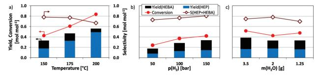
Fig. 5 Influence of process conditions on the reduction of N-(2-hydroxyethyl)succinimide using Ru/C. (Center point for all variations are standard conditions: 150 °C, 150 bar H<sub>2</sub>, 6 h, 750 rpm, 37.5 mg catalyst, 2 g H<sub>2</sub>O solvent.)
