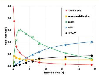
Fig. 2 Concentration-time-profile of the reductive amidation of succinic acid with ethanolamine. (Conditions: 150 °C, 150 bar  $H_2$ , 750 rpm, 1.5 g acid, 1.5 g deionized water, 1 mol. equivalent of amine, 37.5 mg Ru/C) The corresponding reaction network is outlined in Fig. 3. \*HEP = N-(2-hydroxyethyl)-2-pyrrolidone, \*\*HEBA = N-(2-hydroxyethyl)-4-hydroxybutanamide.
