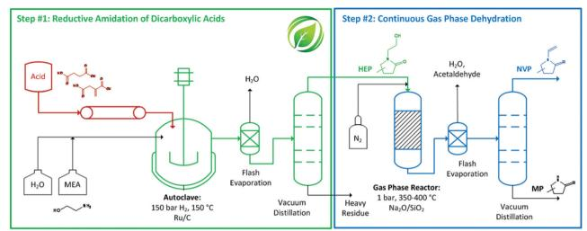
Fig. 1 Schematic of the green value chain proposed herein. Two steps lead from dicarboxylic acids over N-(2-hydroxyethyl)-2-pyrrolidones (HEP) to valuable N-vinyl-2-pyrrolidone monomers (NVP). (MP = methyl-2-pyrrolidone).
