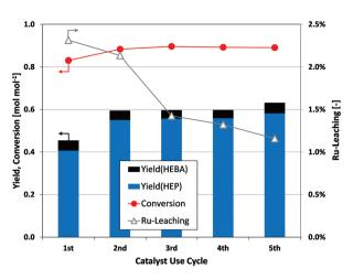
Fig. 6 Assessment of Ru/C catalyst stability by recycling through several N-(2-hydroxyethyl)succinimide reduction batch experiments. (Cond.: 200 °C, 150 bar  $H_2$ , 6 h, 750 rpm; dry catalyst weight for runs 1–5: 50.0 mg, 56.7 mg, 53.5 mg, 52.8 mg and 49.0 mg).
