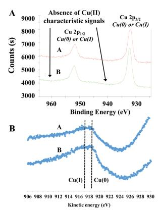
Fig. 4 (A) X-ray photoelectron spectroscopy (XPS) data of Cu8/MgAlO $_x$ -HP (scan A) and Cu8/MgAlO $_x$ -LP (scan B); (B) Auger LMM spectra of Cu8/MgAlO $_x$ -HP (scan A) and Cu8/MgAlO $_x$ -LP (scan B).
