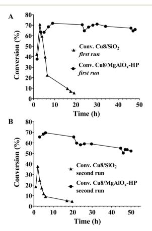
**Fig. 9** (A)  $1^{st}$  run flow Cyrene/LGOL hydrogenation reaction using an oxidized/reduced Cu8/MgAlO<sub>x</sub>-HP and an oxidized/reduced Cu8/SiO<sub>2</sub> material (B)  $2^{nd}$  run flow Cyrene/LGOL hydrogenation reaction using Cu8/MgAlO<sub>x</sub>-HP and Cu8/SiO<sub>2</sub>. Reaction conditions: 353 K, 60 bar H<sub>2</sub>, 1 wt% Cyrene in H<sub>2</sub>O. Flow conditions: Cyrene/H<sub>2</sub>O solution: 0.03 mL min<sup>-1</sup>, H<sub>2</sub> gas: 20 mL min<sup>-1</sup>.
