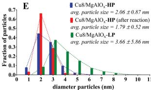
Fig. 3 TEM images of Cu8/MgAlO<sub>x</sub>-HP (A & B); Cu8/MgAlO<sub>x</sub>-LP (C) and Cu8/MgAlO<sub>x</sub>-HP after batch reaction (333 K for 18 h) (D); subfigure E depicts their respective Cu-nanoparticle size distributions. Average (avg.) particle sizes determined from  $\sim$ 1000 particles.
