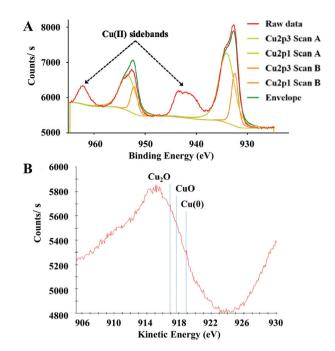
Fig. 6 (A) X-ray photoelectron spectroscopy (XPS) data of recovered Cu8/MgAlO<sub>x</sub>-HP (with peak fitting) and (B) Auger LMM spectra of recovered Cu8/MgAlO<sub>x</sub>-HP.
