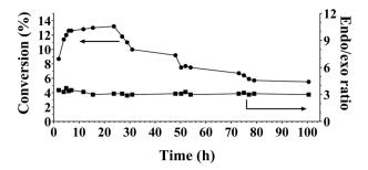
Fig. 8 Activity of reduced Cu8/MgAlOx-HP in flow (353 K, 60 bar  $H_2$ , 5 wt% Cyrene in  $H_2$ O). Flow conditions: Cyrene/ $H_2$ O solution: 0.03 mL min<sup>-1</sup>,  $H_2$  gas: 20 mL min<sup>-1</sup>.
