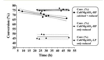
Fig. 7 Comparative activity of "oxidized and reduced" and "sole reduced" Cu8/MgAlO $_x$ -HP in flow (353 K, 60 bar H $_2$ , 1 wt% Cyrene in H $_2$ O). Flow conditions: Cyrene/H $_2$ O solution: 0.03 mL min $^{-1}$ , H $_2$  gas: 20 mL min $^{-1}$ .
