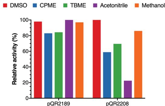
**Fig. 5** Effect on yield of **18b** with various co-solvents (10% final concentration). The reaction conditions used were the same as those indicated in Fig. 4, all reactions were performed in triplicate and standard deviations were <8%.
