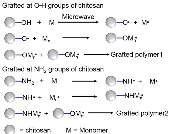
Fig. 3 Grafting mechanism of chitosan under microwave irradiation. Reproduced from ref. 60. Copyright (2004), with permission from Wiley-VCH.
