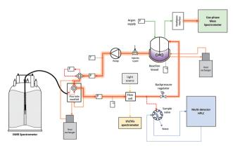
Fig. 2 Schematic of the *operando* analytical recirculating flow setup (for details see the ESI†).
