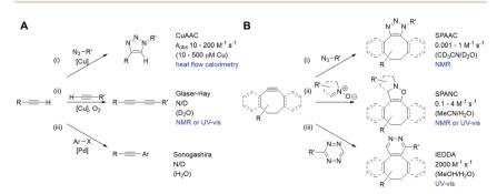
Fig. 1 Bioorthogonal reactions of terminal alkynes (A) and strained alkynes (B), with approximate rate constants in aqueous based media (N/D = not determined). (A) (i) Copper(I) catalysed azide-alkyne cycloaddition (CuAAC);23 (ii) Glaser-Hay reaction;24 (iii) copper-free Sonogashira reaction.<sup>25</sup> (B) (i) Strain-promoted azide-alkyne cycloaddition (SPAAC);26 (ii) strain-promoted alkyne nitrone cycloaddition (SPANC);26 (iii) inverse electron demand Diels-Alder (IEDDA).27
