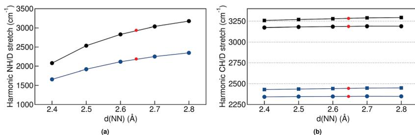
Fig. 6 Selected harmonic stretch frequencies for *trans* structures where all degrees of freedom were optimized except for  $d(\text{NN})$ . In (a) we show the NH and ND stretch frequencies for Pc-*d0* (black) and Pc-*d2* (blue) as a function of  $d(\text{NN})$ . In (b) we show the CH and CD stretch frequencies for Pc-*d0* (black) and Pc-*d12* as a function of  $d(\text{NN})$ . The red dots represent the values for the relaxed structure.
