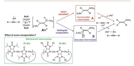
Scheme 1 Proposed mechanism for nucleophilic addition to alkyne catalysed by gold(I) and the structures of the studied bambusurils.
